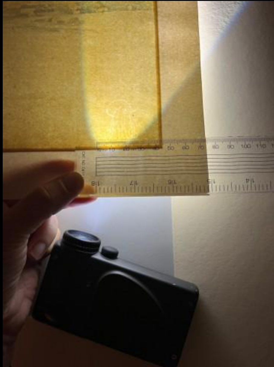
Former method of measuring and photographing watermarks
