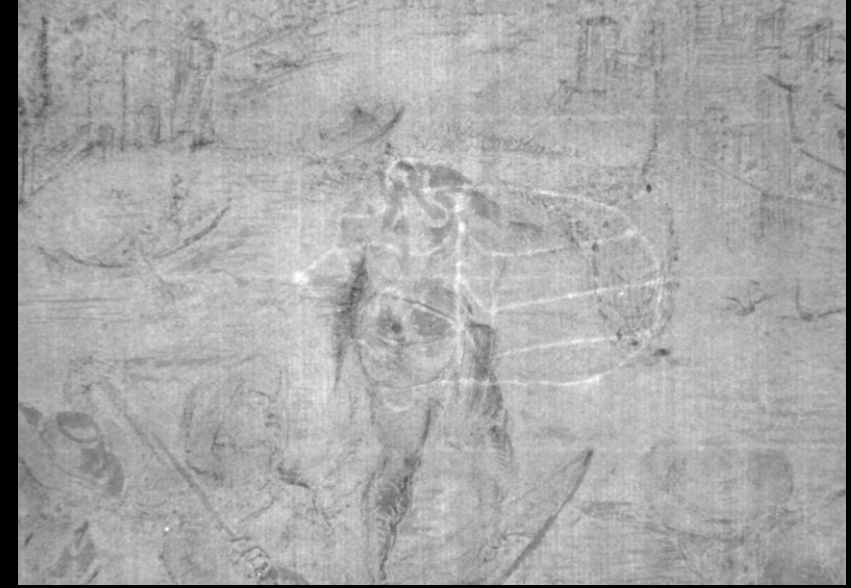
Watermark taken with VSC using transmitted light and infrared
